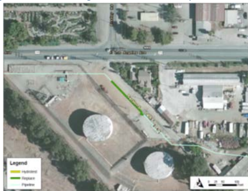
Figure 12: Satellite Image of L-406 Section 5 Replacement Project
