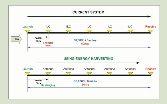
In 2019, the project team demonstrated an onboard energy harvesting module that enabled an Explorer model in-line inspection robot to avoid the need for in-line charging and dramatically reduce inspection times.
