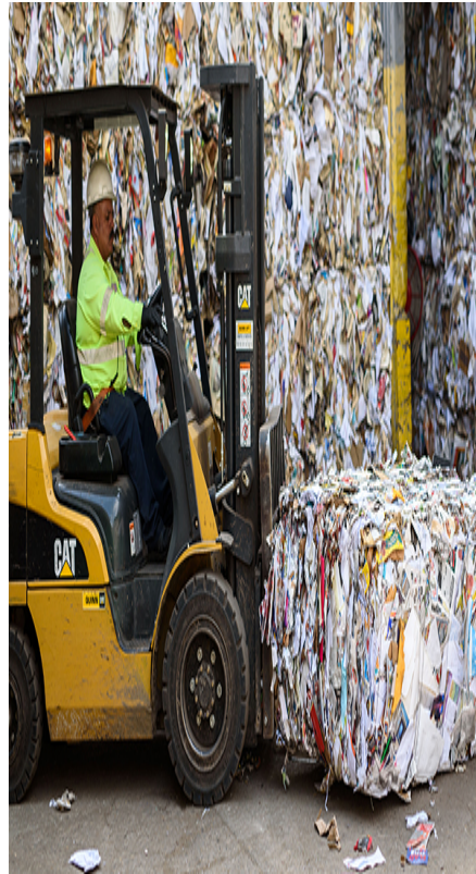
11. Workers take sorted recyclables and condense the material into large bales.
