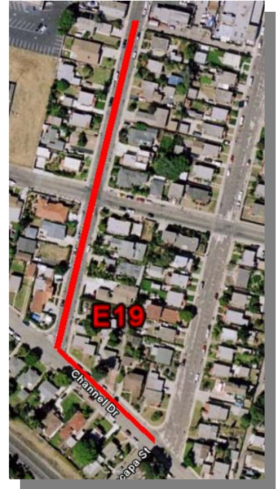
Project E19 replaces 1,040 linear feet of 6- and 8-inch sewers on Santa Cruz Street and Channel Drive.
