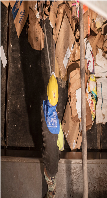
10. A worker uses a specially designed tool to clear out any noncardboard recyclables along bailing conveyors.
