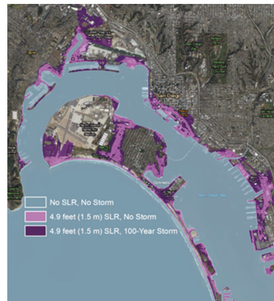
The CoSMoS tool permits assessment of flood risk for all parts of California. This image shows the San Diego Harbor with a 4.9 foot sea level rise and with or without a 100-Year storm.
