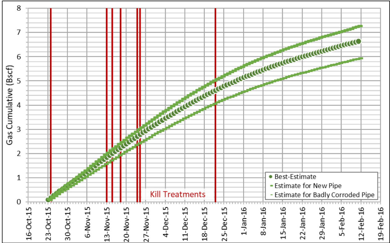
Figure 125: SS-25 Leak Cumulative Estimate (October 23 to February 11)
