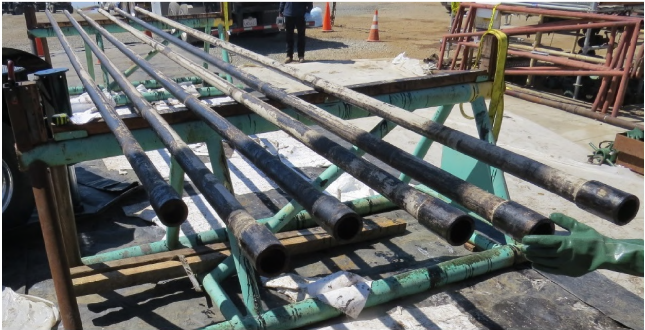
Figure 27: Tubing Joints on the SS-25 Pipe Rack
