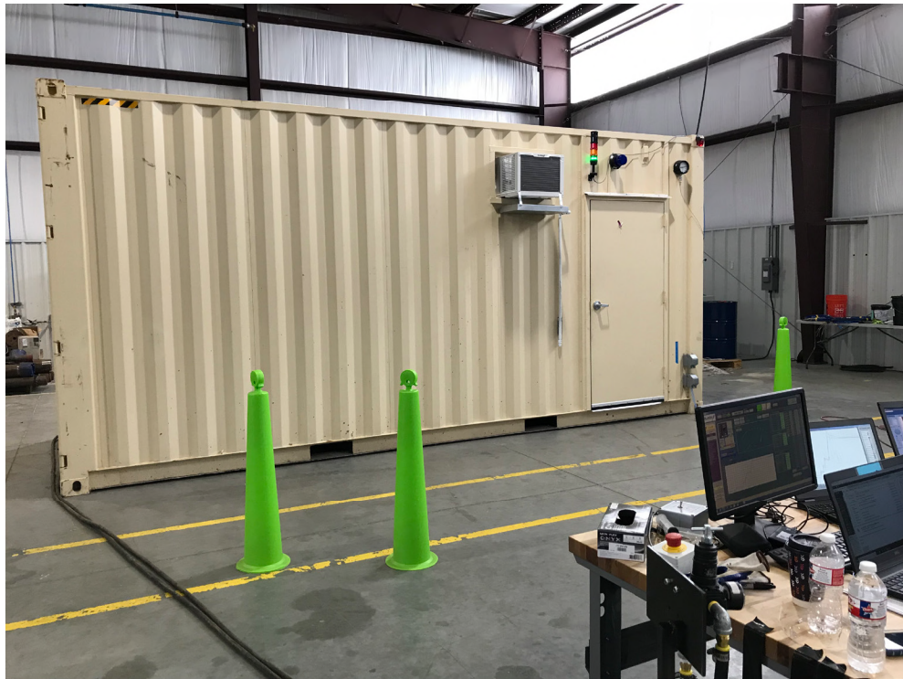
Figure 10: Conex Trailer Used for Connection Testing
