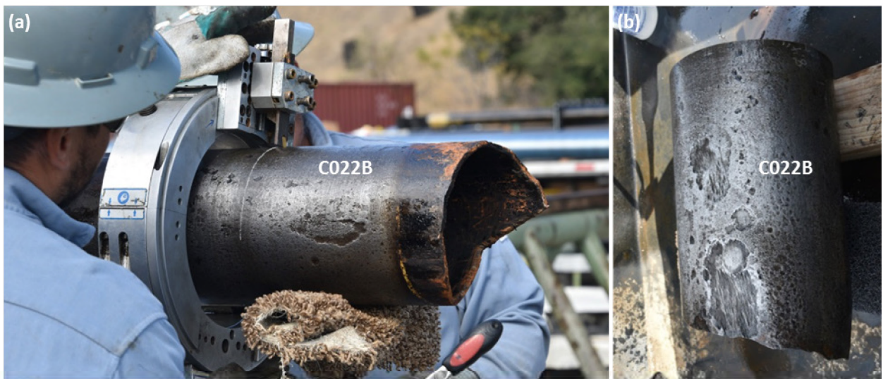
Figure 59: Fracture Surface During (a) Extraction from C022 and After (b) Cleaning with Sentinel 909
