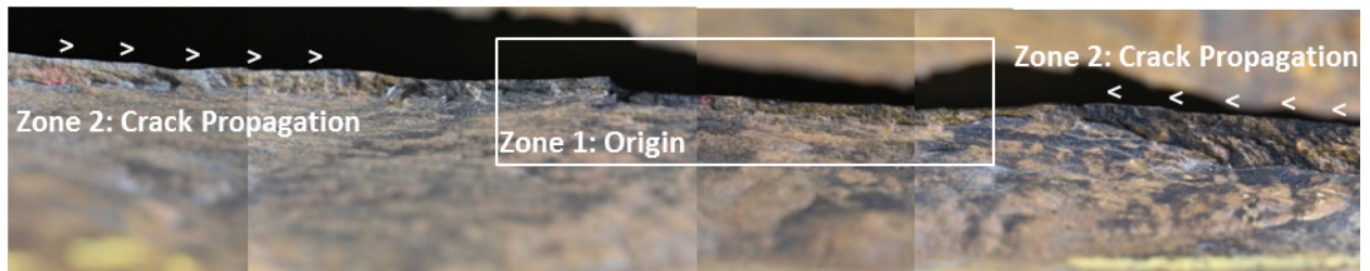
Figure 82: Close-up of Zone 1 and Zone 2 of the Axial Rupture
