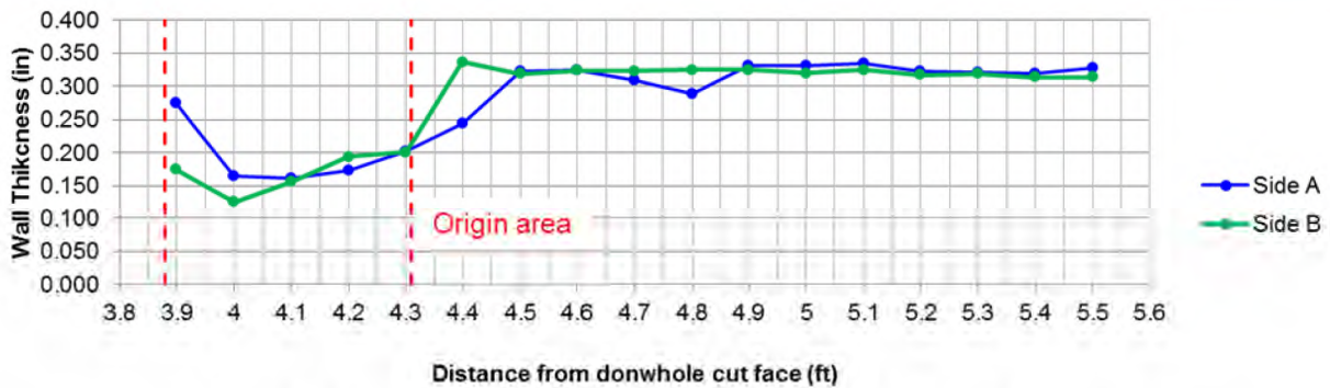
Figure 83: Remaining Wall Thickness Measurements of Axial Rupture
