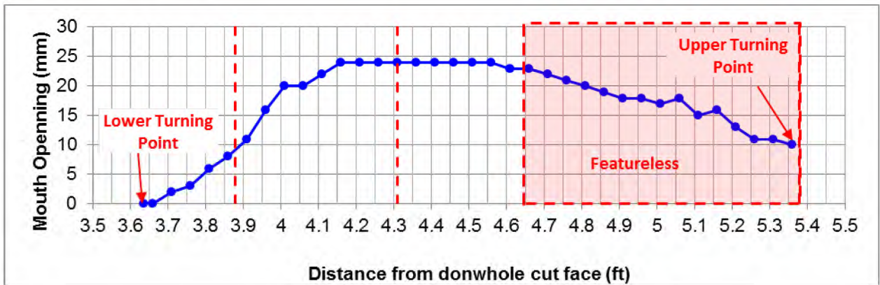
Figure 85: Plot of Fracture Surface Mouth Opening Versus Axial Position
