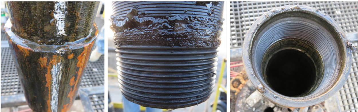
Figure 23: T155–T156 Connection Before and After Breakout
