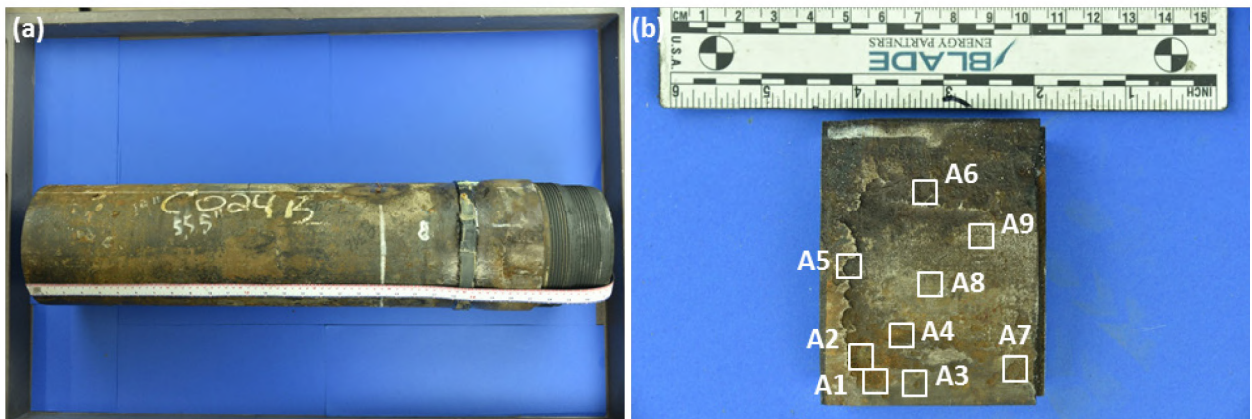
Figure 253: (a) Connection C024B and (b) Type III Corrosion Specimen C024B1B
