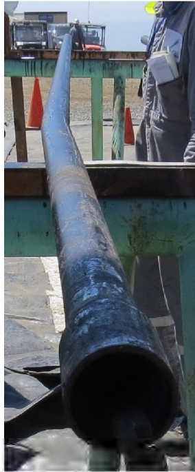
Figure 8: 2 7/8 in. Tubing Joint 116 After Extraction
