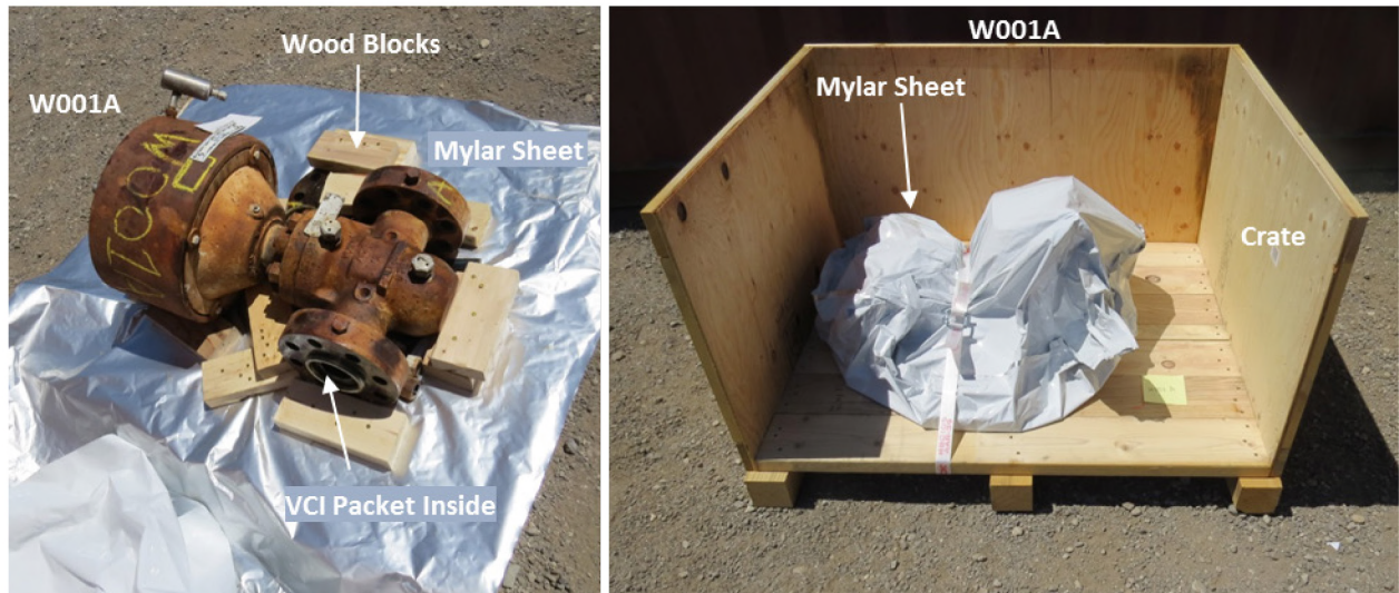
Figure 22: Crating of Wellhead Component W001A
