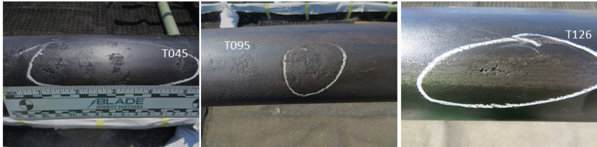
Figure 32: Examples of Minor Metal Loss
