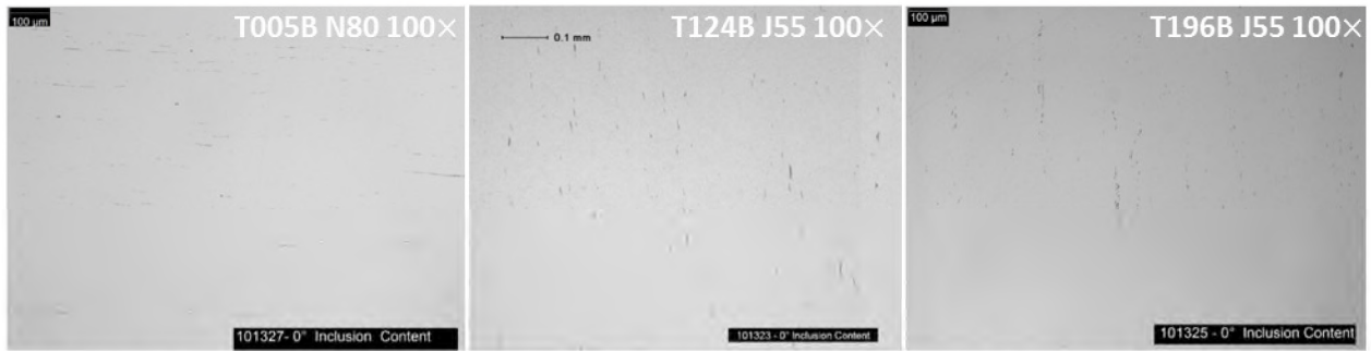
Figure 309: Microcleanliness Micrographs for (a) T005B, (b) T124B, and (c) T196B Taken at 100×
