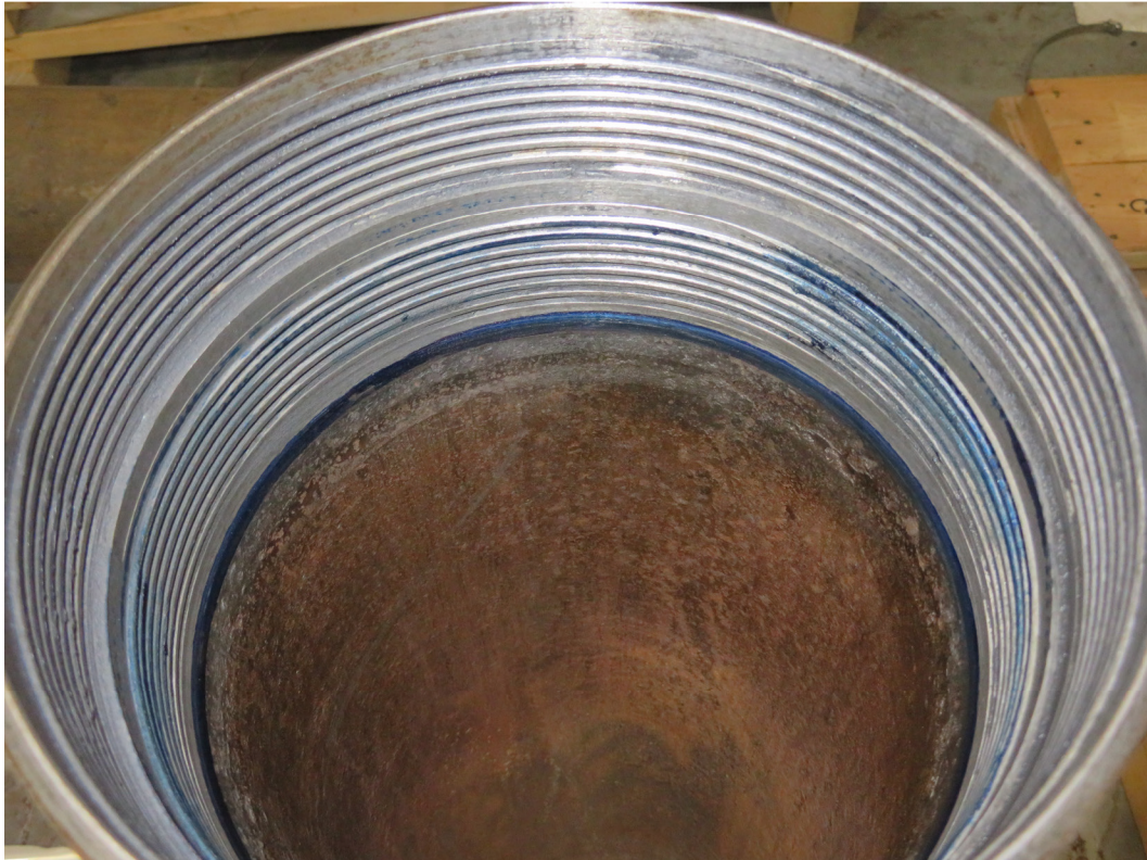
Figure 20: Representative Full Blueing Transfer on C002B
