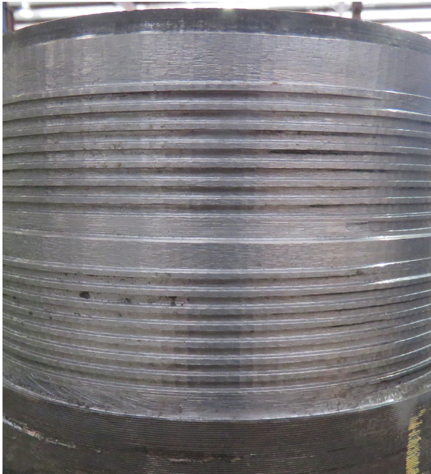
Figure 5: C001B Pin Threads Condition after Cleaning
