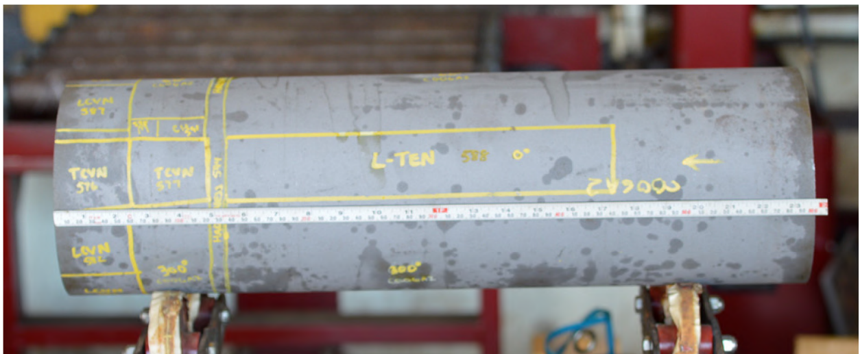
Figure 281: Material Testing Layout for Specimen C006A2
