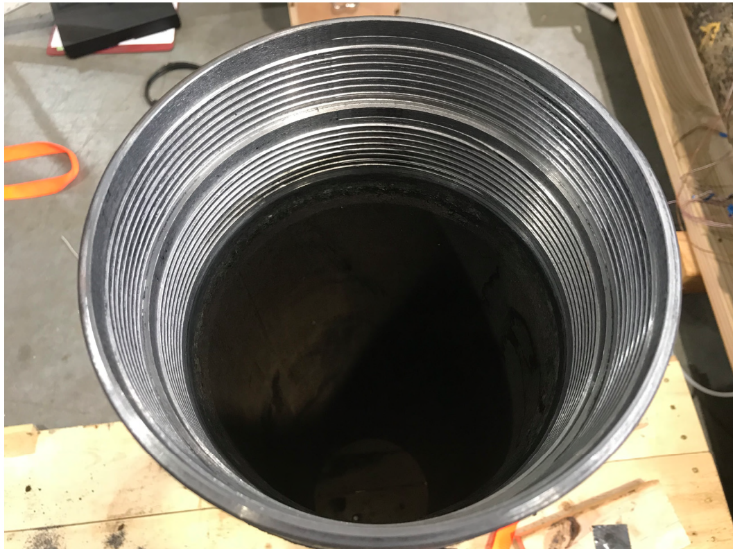
Figure 19: Representative Box Condition after Break out and Cleaning
