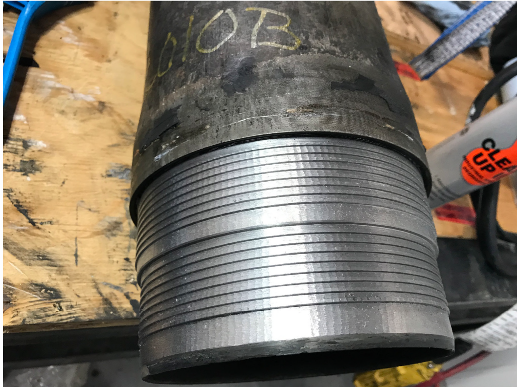
Figure 18: Representative Pin Condition after Break out and Cleaning
