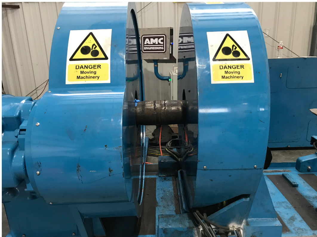
Figure 17: Breaking Out a Connection with the Horizontal Bucking Machine
