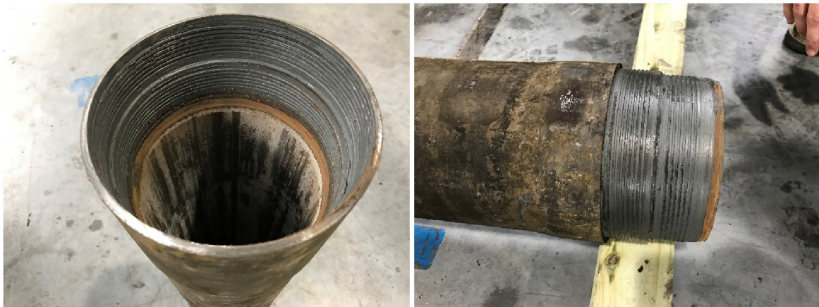
Figure 12: Photos of a 7 in. Speedtite Connection Showing the Box and Pin
