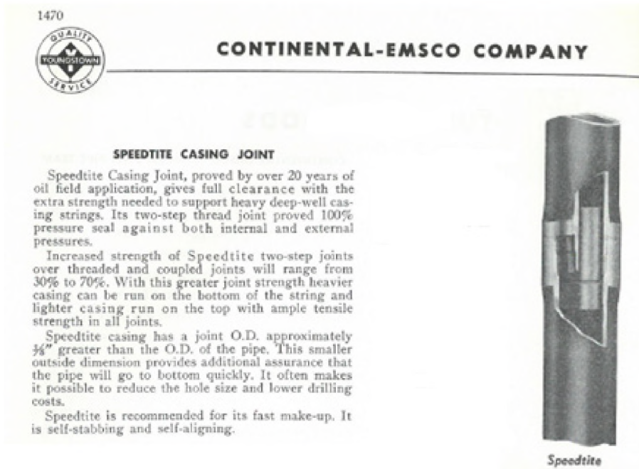
Figure 11: Information on the Speedtite Connection from the 1960 Composite Catalogue
