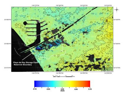
Figure 19: Vertical deformation from March 6, 2010 to June 10, 2010.
