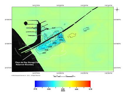
Figure 23: Vertical deformation from March 1, 2011 to June 29, 2011.
