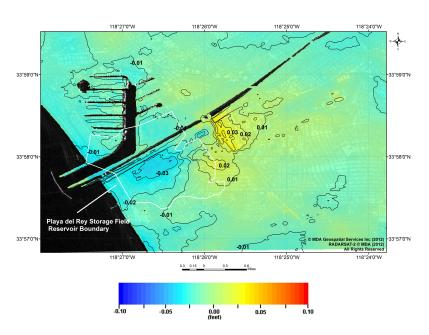
Figure 27: Vertical deformation from March 19, 2012 to June 23, 2012.
