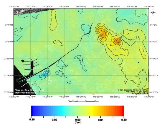
Figure 6: Playa del Rey Gas Storage Field AOI and surrounding area. Color representation of the vertical deformation product from March 14, 2013 to June 18, 2013 superimposed on SAR image with 0.01 ft contours. In this representation, blue corresponds to subsidence and red indicates uplift.
