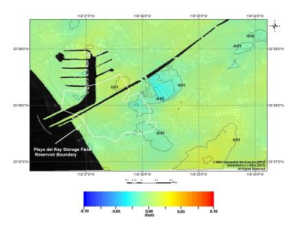
Figure 28: Vertical deformation from June 23, 2012 to September 3, 2012.
