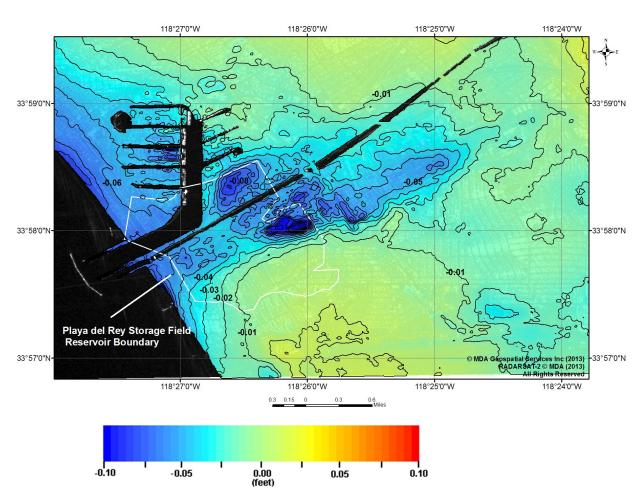
Figure 10: Zoom-in of Playa del Rey Gas Storage Field AOI and surrounding area. Cumulative vertical deformation from May 27, 2008 to June 18, 2013, with 0.01 ft contours.
