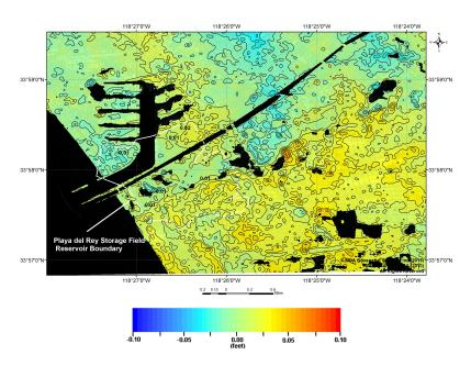
Figure 16: Vertical deformation from June 15, 2009 to September 19, 2009.
