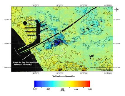
Figure 15: Vertical deformation from March 11, 2009 to June 15, 2009.
