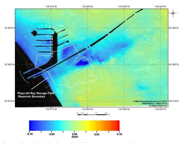
Figure 11: Playa del Rey Gas Storage Field AOI and surrounding area. Color representation of the cumulative vertical deformation from May 27, 2008 to June 18, 2013 superimposed onto SAR image.
