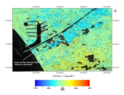
Figure 12: Vertical deformation from May 27, 2008 to August 31, 2008.
