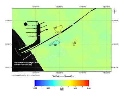
Figure 24: Vertical deformation from June 29, 2011 to September 9, 2011.
