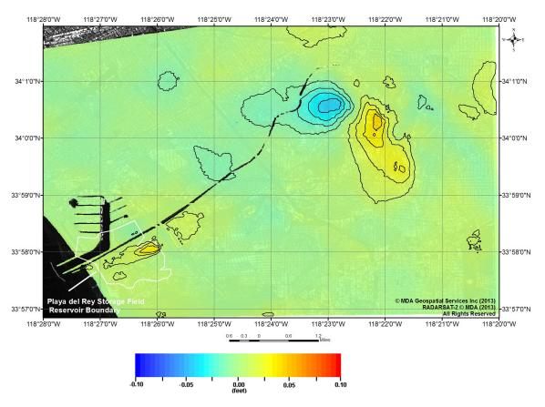
Figure 3: Playa del Rey Gas Storage Field AOI and surrounding area. Color representation of the vertical deformation product from December 8, 2012 to March 14, 2013 superimposed on SAR image with 0.01 ft contours. In this representation, blue corresponds to subsidence and red indicates uplift.
