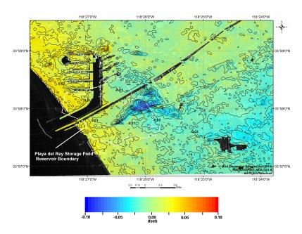
Figure 20: Vertical deformation from June 10, 2010 to September 14, 2010.
