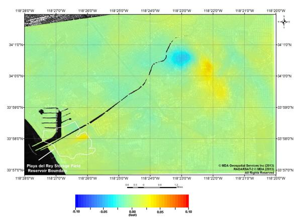
Figure 2: Playa del Rey Gas Storage Field AOI and surrounding area. Color representation of the vertical deformation product from December 8, 2012 to March 14, 2013 superimposed on SAR image without contours. In this representation, blue corresponds to subsidence and red indicates uplift.
