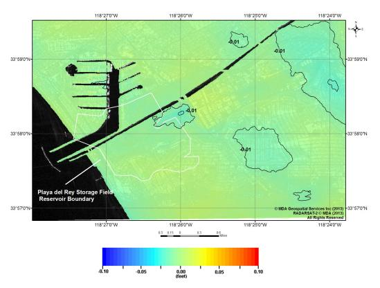
Figure 8: Playa del Rey Gas Storage Field AOI and surrounding area. Color representation of the cumulative vertical deformation from December 8, 2012 to June 18, 2013 superimposed onto SAR image.
