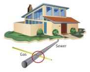
If an exterior sewer line blockage may be near or caused by a natural gas pipeline that has penetrated the sewer line, please call Southern California Gas Company (SoCalGas®) at **1-800-427-2200** before you attempt to clear the line. We will respond by phone and tell you if it is safe to clear, or visit the site at no charge to verify.
