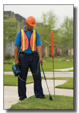
The **HEATH** Detecto Pak-Infrared (DP-IR<sup>™</sup>) is a highly advanced technology capable of detecting methane without false alarming on other gases. The DP-IR is the latest generation of leak survey instruments from **HEATH** that will greatly improve the productivity and safety of a walking/mobile survey.
