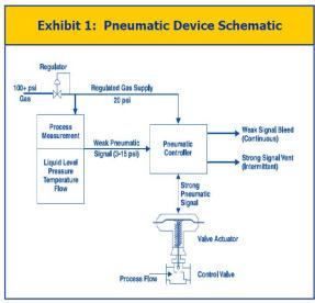
Figure 4: Pneumatic Device Schematic<sup>61</sup>
