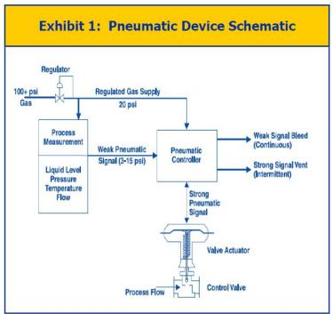
Figure 2: Pneumatic Device Schematic<sup>61</sup>
