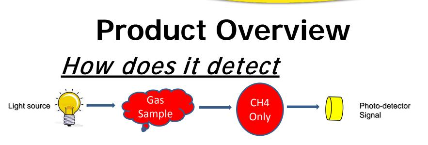
PMD uses an infrared a light source that is of the same frequency that methane gas will absorb.
