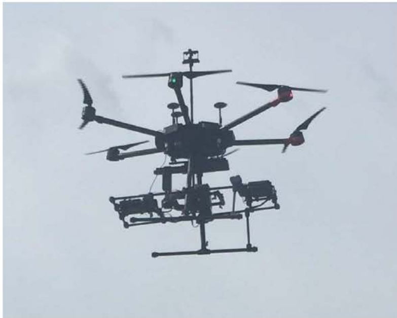
Figure 1. SoCalGas sUAS with dual methane sensors
