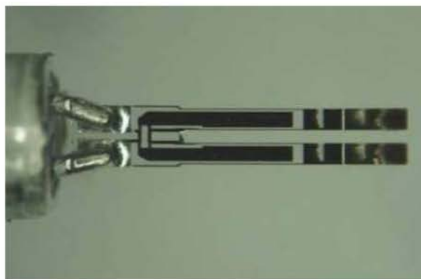
Turning Fork Used in Micro-Resonator
