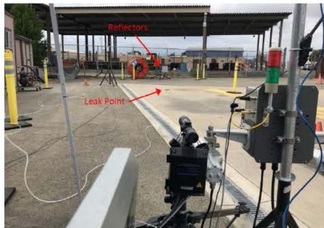
Figure 1. Simulated Field Testing Open Path Units Aimed at Reflectors
