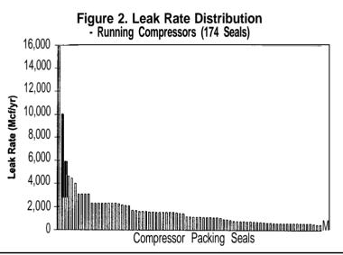
piece leakage totaled 19,930 Mcf/y, approximately five times more than the packing cup leakage alone. Table 3 illustrates the distribution in leakage from packing cup and distance piece vents on running compressors. Measurements conducted at two sites during this study, as well as at six private client facilities, indicate that distance piece leakage typically accounts for approximately 30% of the total leakage from the compressor packing seals.
