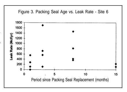
measurement (\$3,400/yr). Furthermore, there does not seem to be an observable trend in leak growth with packing age. The average packing seal leak rate after 1,3,8 and 15 months is 230, 770, 770, and 165 Mcf/yr, respectively. Since most sites do not seem to keep a detailed record of rod packing replacement schedules, further data regarding the age of rod packings is scarce.
