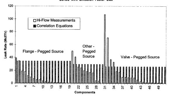
Figure 2. Comparison of Leak Rate Estimates Using Emission Factors and Hi-Flow Measurements
