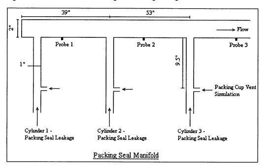
Figure 4. Test Manifold for Monitoring Rod Packing Leakage with Hot Wire Anemometer
