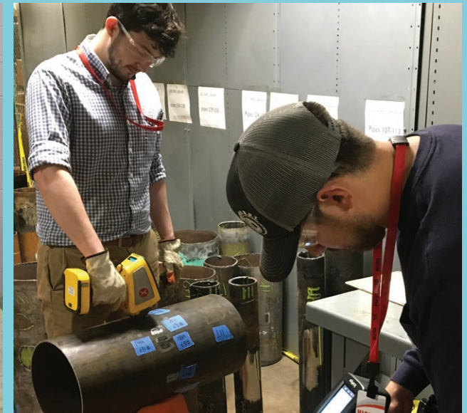
Project team members first lab-tested the samples for yield strength, ultimate tensile strength, steel chemistry, grain size, hardness, and in a subset of 30 samples, material fracture and Charpy toughness.
