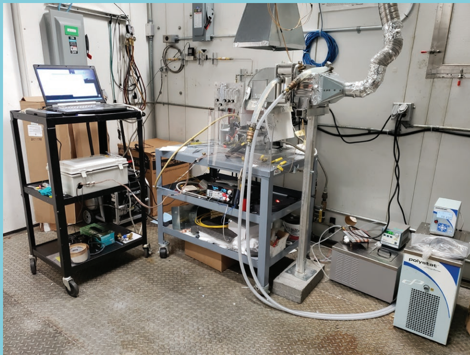
Thermal cycling test of the heterogeneous burner in the presence of 50% hydrogen. Also shown is the cold and hot restart of the burner.
