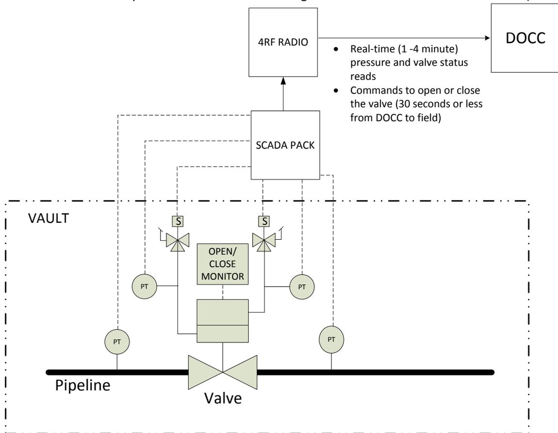
**Figure 8: Remote Control Valve Schematic**
