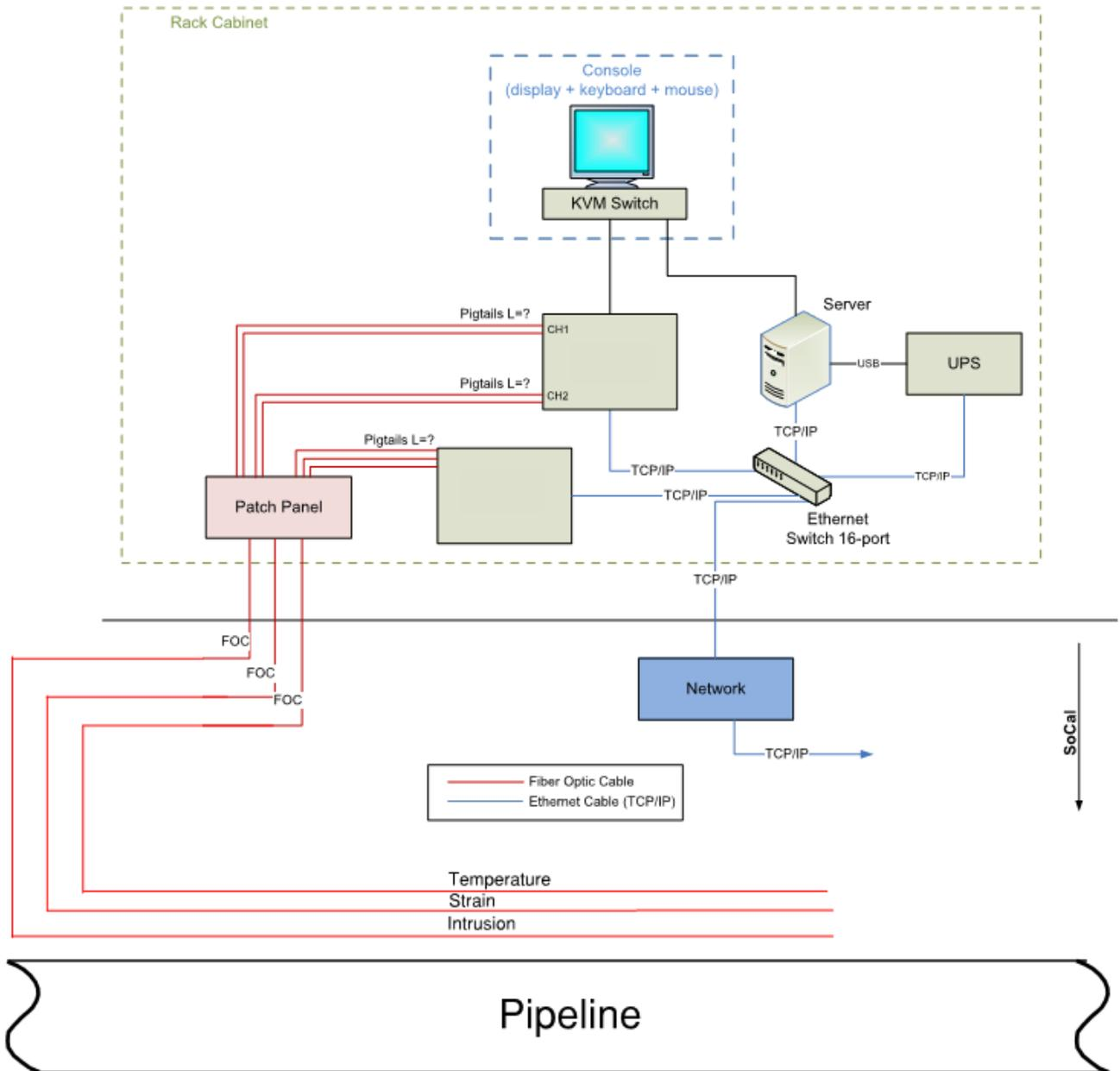
Below you will find the typical configuration of a fiber monitoring station rack which holds the servers, instruments and uninterruptible power supply.
