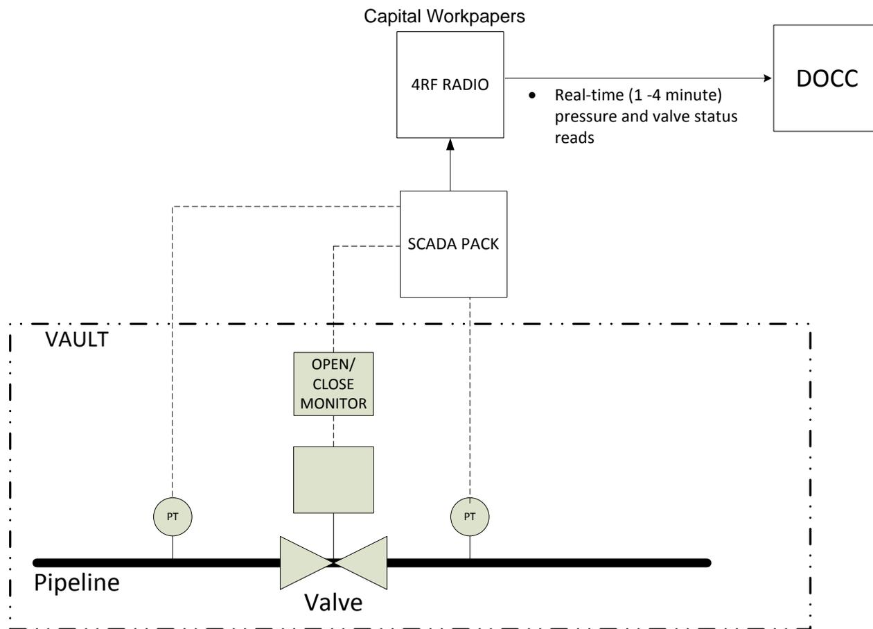
**Figure 6: Real-time Monitoring Site Schematic**
