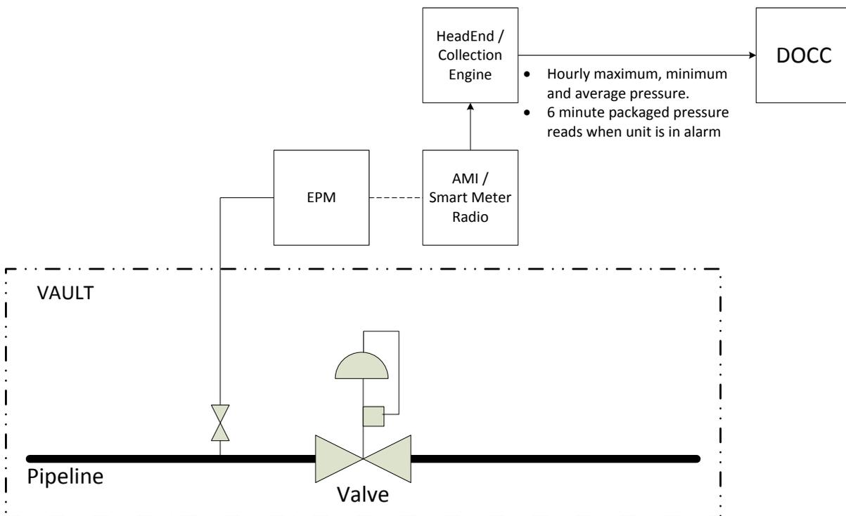
**Figure 3: EPM Site Schematic**
