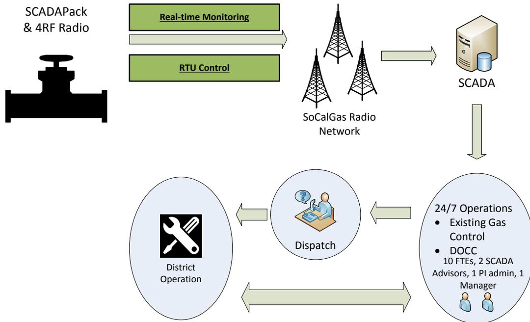
**Figure 2: Real-time Monitoring and Control Sites**
