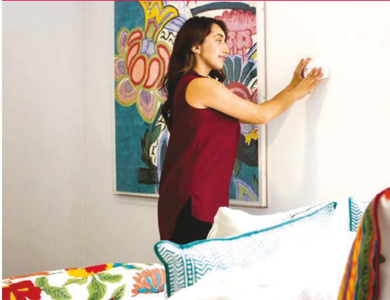
monoxide alarm. Only carbon monoxide alarms that are approved by the California State Fire Marshall and have the Underwriter's Laboratories (UL) Certification may be used. They are available at your local hardware and home improvement stores.
