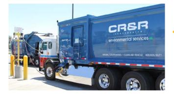
Near-zero-emissions natural gas engines reduce NOx emissions up to 90 percent and GHG emissions up to 80 percent compared to diesel.<sup>53</sup>
