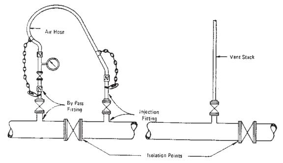
Figure 2 - Arrangement for Directly Purging Pipelines into Service.
