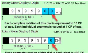
Each complete rotation of this dial is equivalent to 100 CF of gas. Each individual segment is valued at 10 CF of gas.
