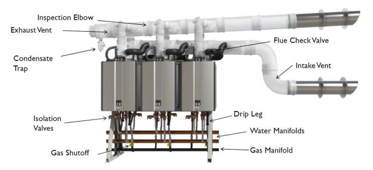
Just add 120Vac power, vent, connect water and gas and you're ready for hot water!
