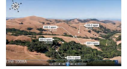
Aviation Services used the sUAS to conduct a virtual "job walk" along Line 1008A, a pipeline with many hidden and hazardous spans.
