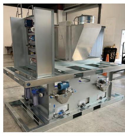
The innovative A/C system incorporates heat recovered from gas-fueled CHP units—including fuel cells—via a load-shifting thermochemical energy-storage system that uses a liquid desiccant to store energy.
