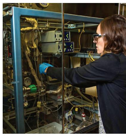
A research team from PNNL and WVU developed and demonstrated a thermocatalytic decomposition process to convert methane into hydrogen at a bench scale. The process also yields a high-value solid carbon co-product suitable for a variety of manufacturing applications.
