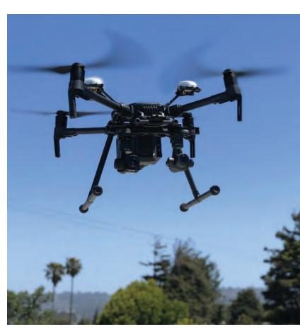
The SoCalGas Aviation Services Group operates small Unmanned Aerial Systems for use in the inspection of gas facilities, meters, and pipelines that are remote or difficult to access.
