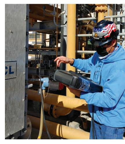
To verify compliance with emission limits, plant and facility operators conduct expensive and complicated tests using EPA Reference Methods with analyzers in a large trailer or truck or handheld, electrochemical analyzers.
