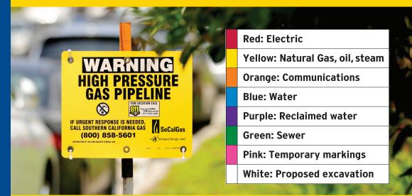
High-visibility markers, like this, identify the general location of major pipeline routes. Contact **811** for accurate pipeline location markings.
