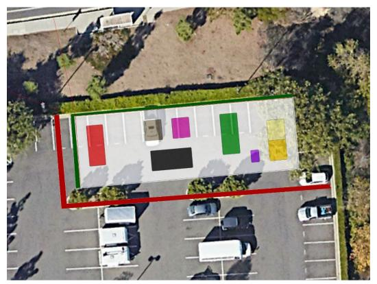
**Equipment Type** Color Electrolyzer Green Orange SCADA Building Yellow Storage Shed Hydrogen Storage Red Chiller Unit Purple Gas Composition Analyzer Brown Blending Skid Black Hydrogen Compressor Pink
