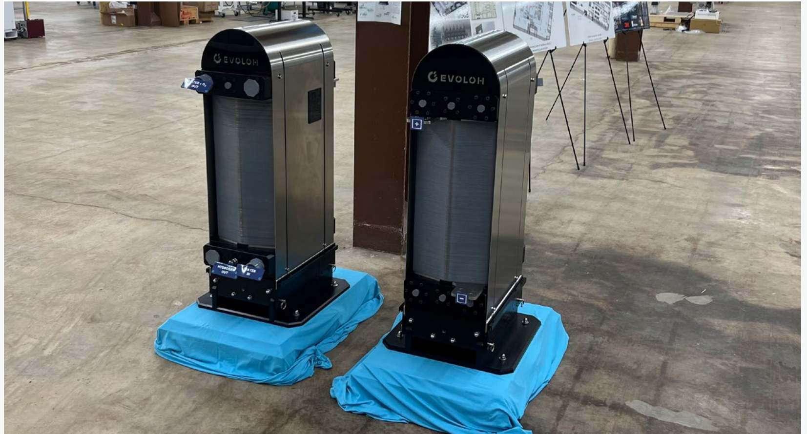
EVOLOH's megawatt-scale advanced liquid alkaline electrolyzer stack.
