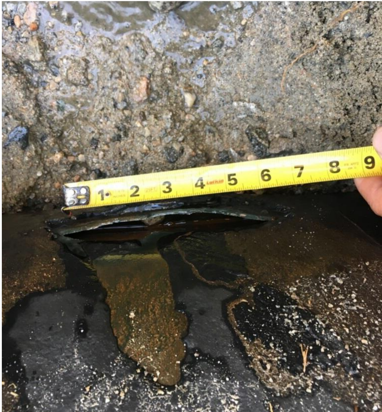
Figure 8: 6-inch Rupture of Hydrotest 2
