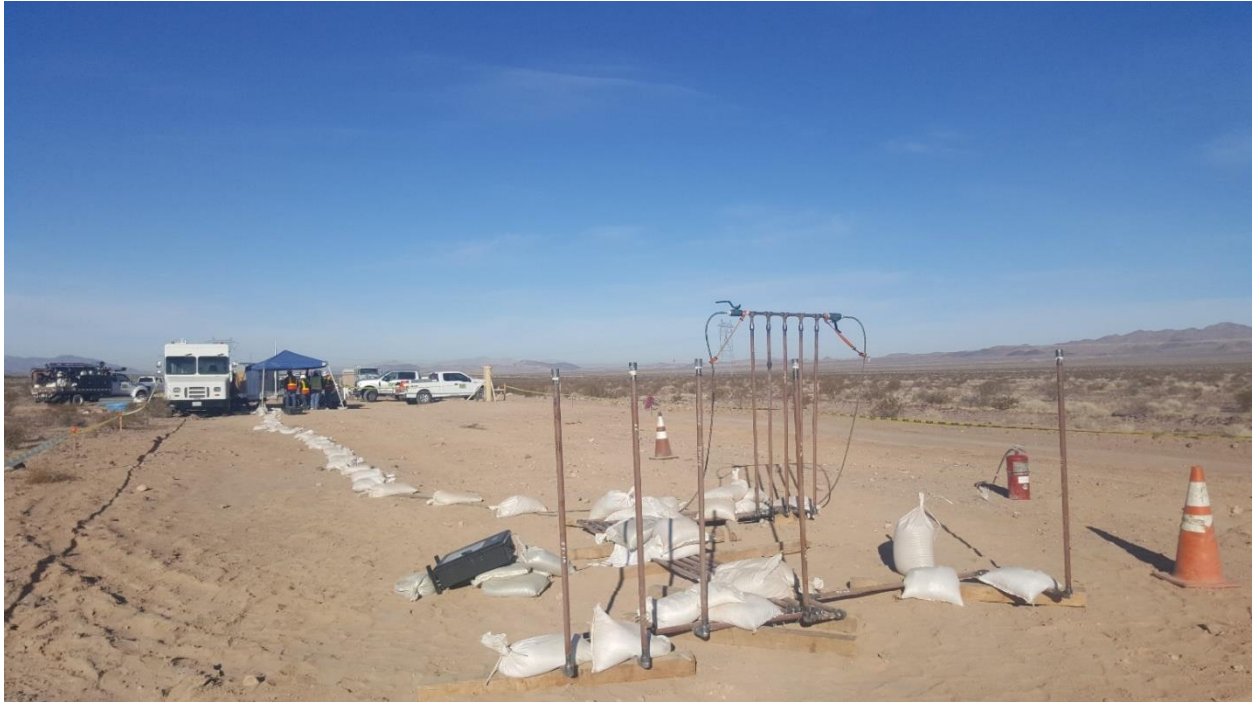
Figure 4: Nitrogen Test for New Instrument Piping
