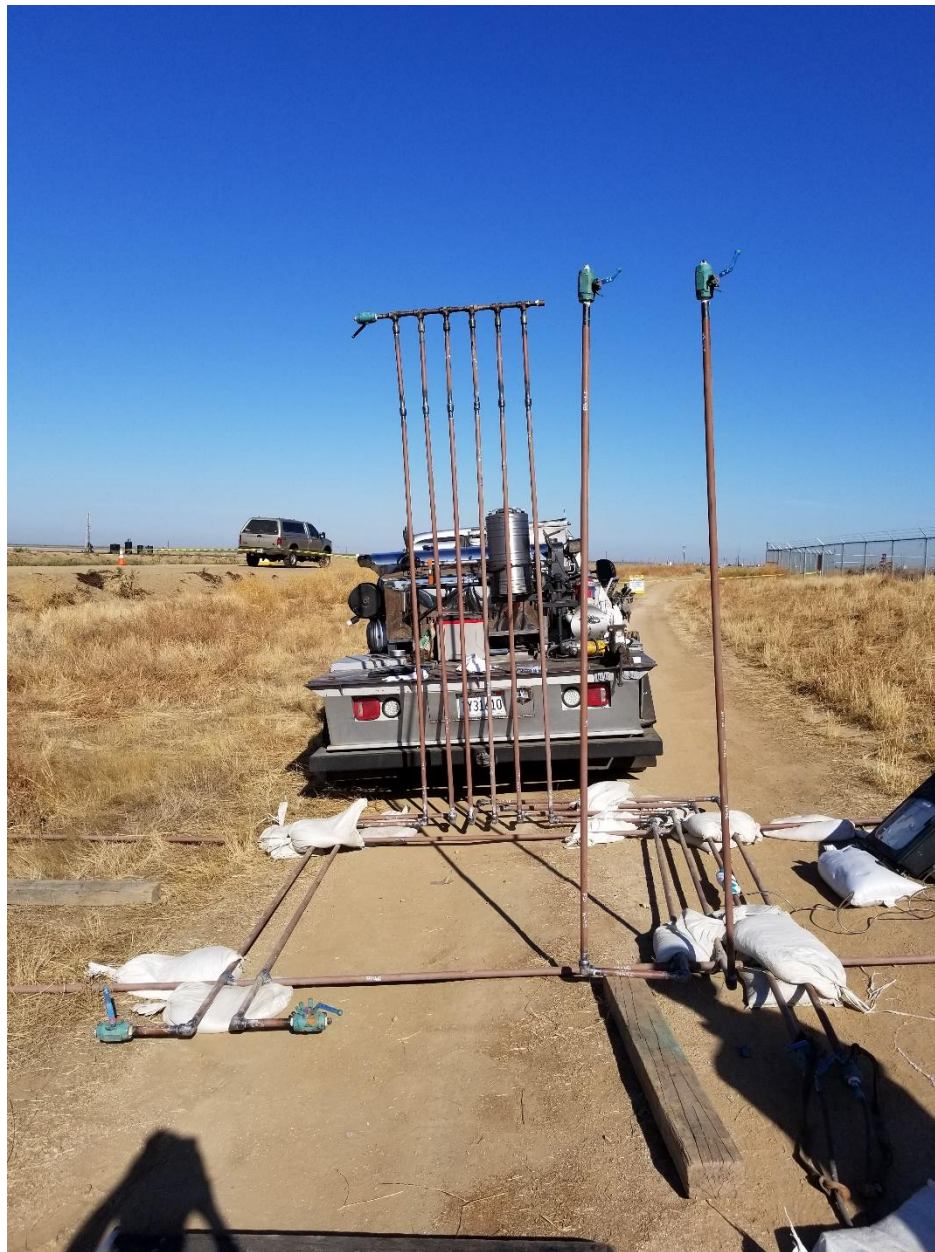
Figure 4: Setup for Instrument Piping Pressure Test
