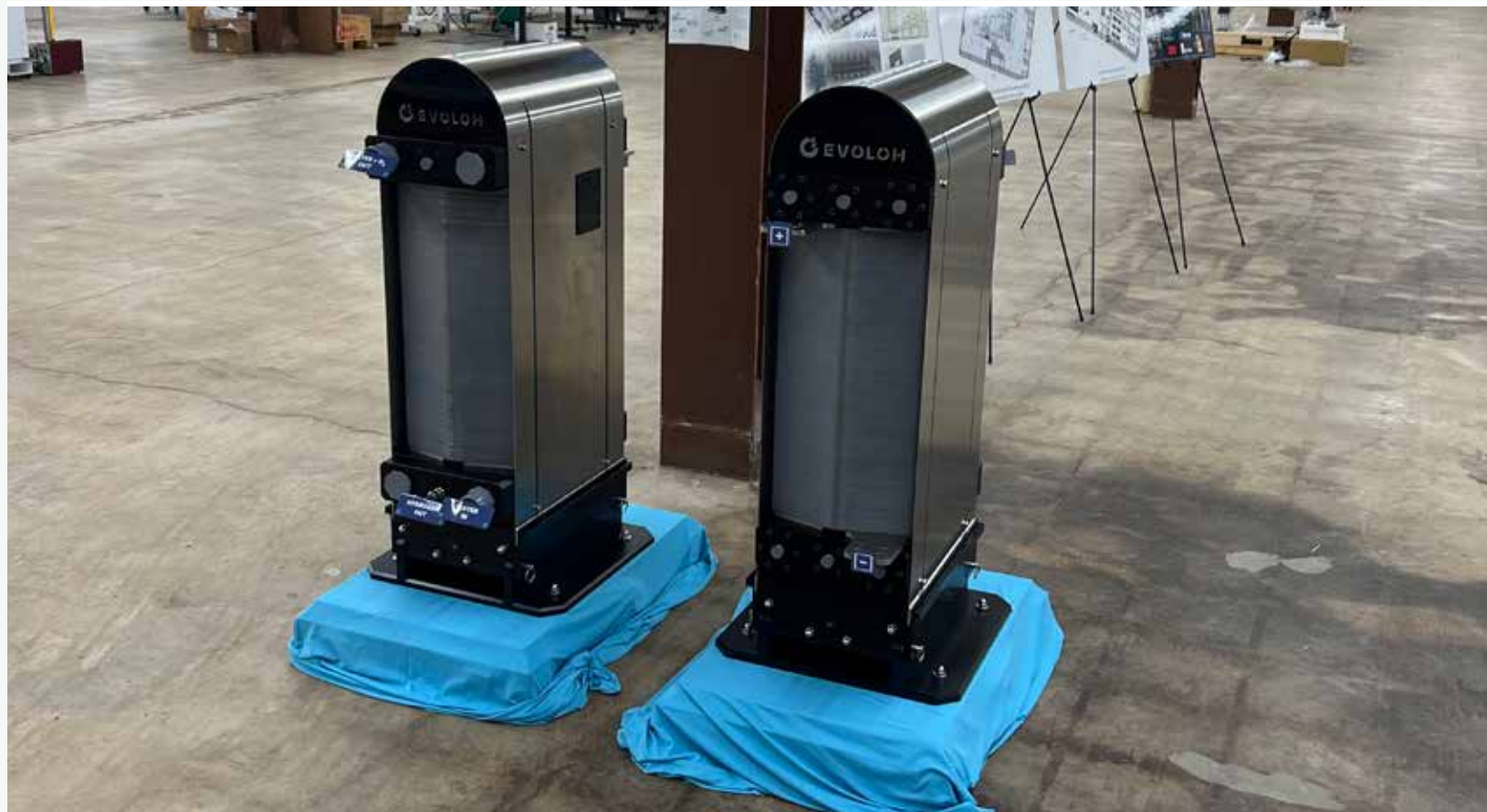
EVOLOH's megawatt-scale advanced liquid alkaline electrolyzer stack.
