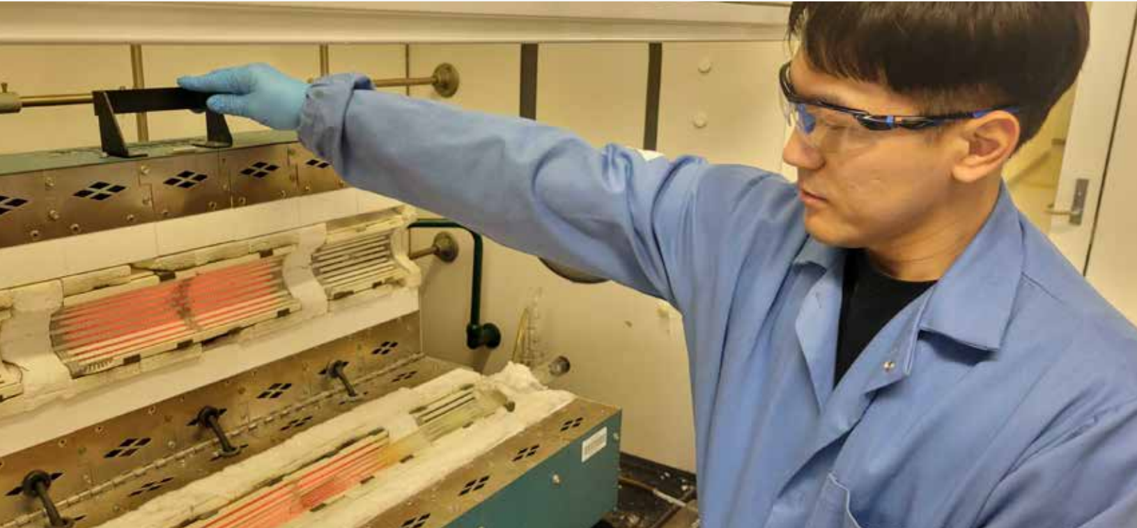
On a project exploring reducing hydrogen compression costs, Caltech Staff Scientist Mason Jang uses a tube furnace to synthesize the molybdenum carbide catalyst.
