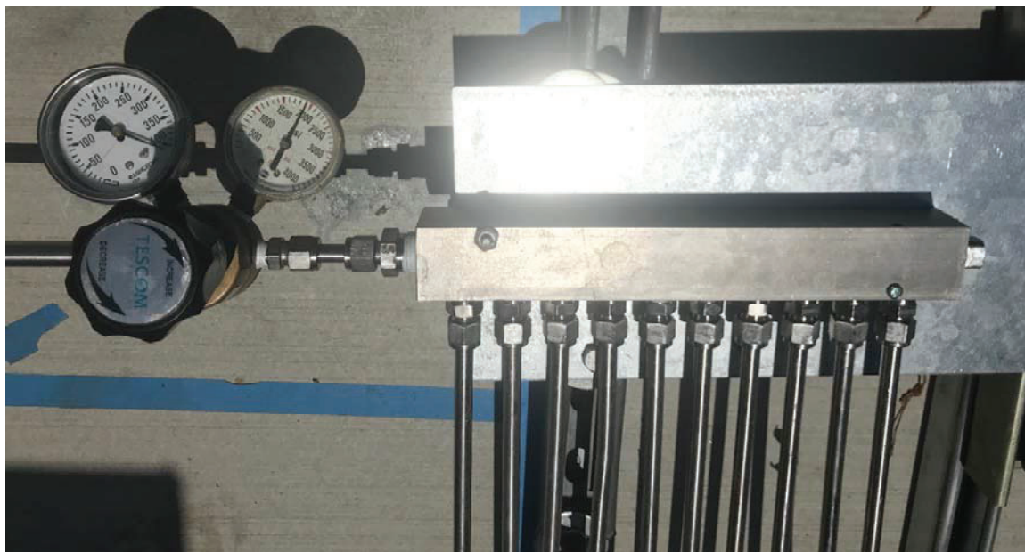
Figure 98. Pressure regulator and cylinder manifold used in high throughput hydrogen testing.
