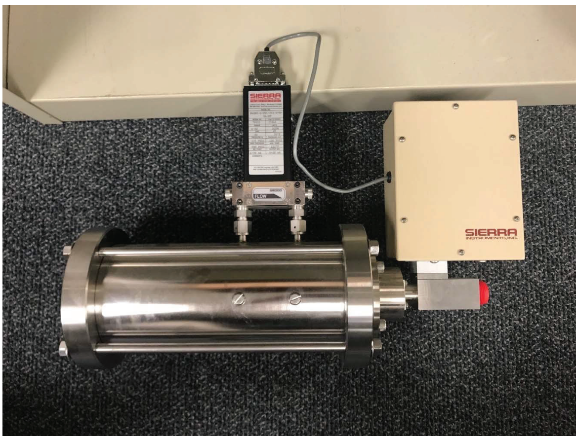
Figure 96. Sierra Hi-Trak 840 mass flow controller utilized in high throughput hydrogen injection testing.
