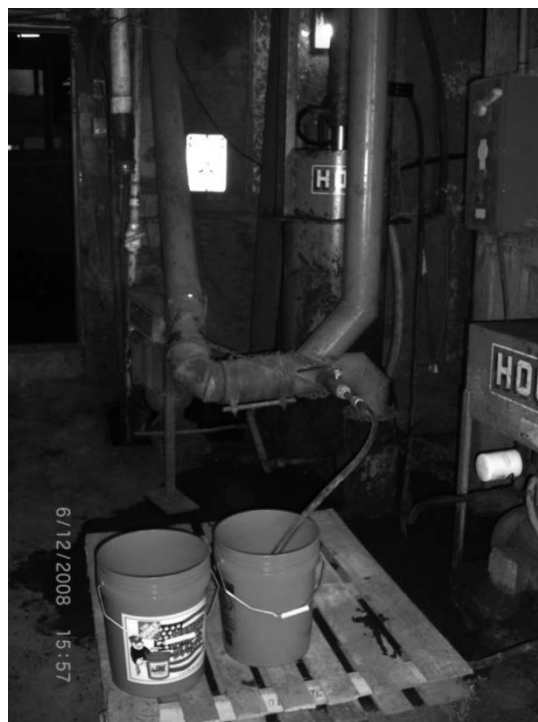
Photo 3-3— EMG Sampling of the Raw Manure Stream Fed into the AA Dairy Digester
