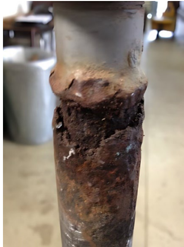
Figures 2 and 3. Anodeless Riser After Remediation
