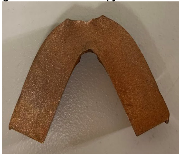
Figure 109: Photo of Charpy Tested Cu Alloy
