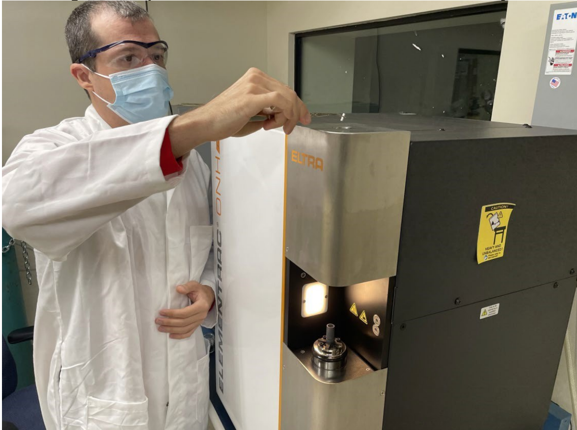
Figure 85: Operation of the Elementrac ONH Elemental Analyzer
