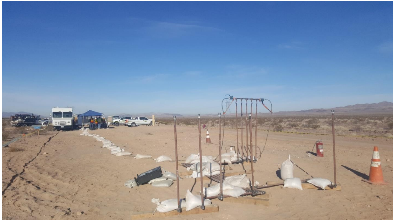
Figure 4: Nitrogen Test for New Instrument Piping
