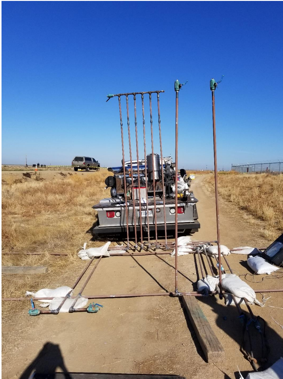
Figure 4: Setup for Instrument Piping Pressure Test
