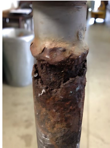
Figures 2 and 3. Anodeless Riser After Remediation
