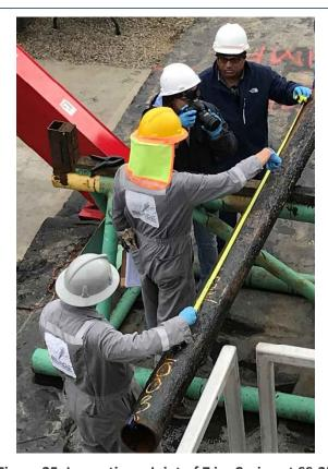
Figure 25: Inspecting a Joint of 7 in. Casing at SS-25
