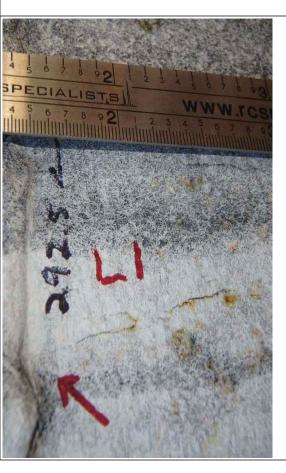
Description: Surface lamination detected at 292.5 degrees below girth weld
