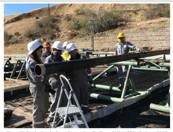
Figure 29: Conducting the Second Inspection of a Cleaned Joint of 7 in. Casing at PS-20
