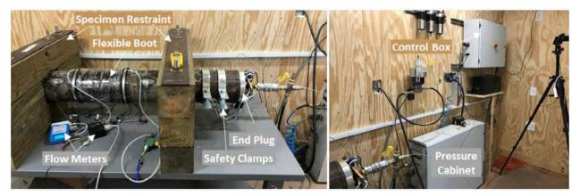
**Figure 22: Connecting Test Setup**
