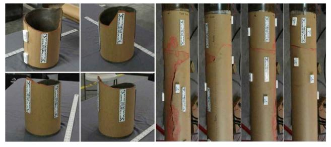
Figure 12: Completed Paper Reconstruction of C022B and C023A1
