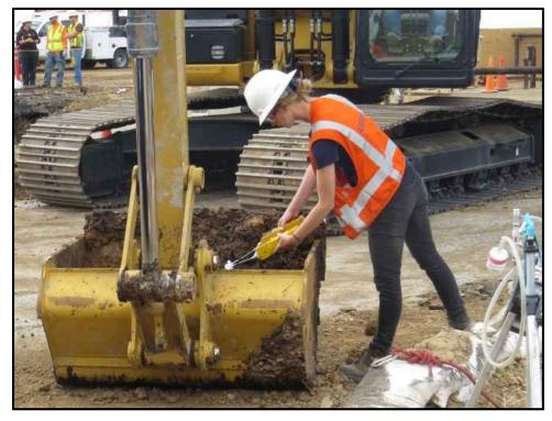
Figure 36: AECOM Sniff Testing for Isobutylene (Correlated to Hexane for SCAQMD Rule 1166)
