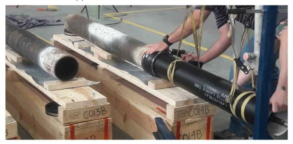
Figure 13: Laserstream Connection Scan
