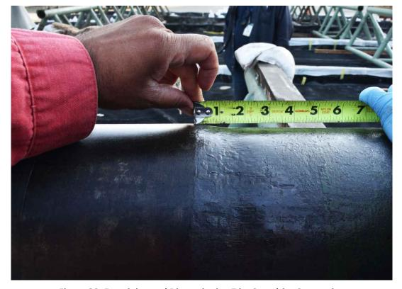
Figure 30: Examining and Dimensioning 7 in. Speedtite Connection
