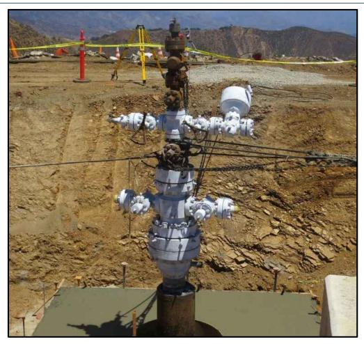
Figure 57: Cleaned Wellhead, Completed Non-Destructive Evaluation
