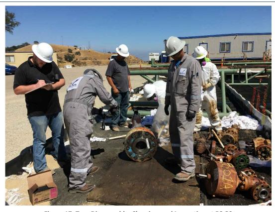
Figure 17: Tree Disassembly, Cleaning, and Inspection at PS-20
