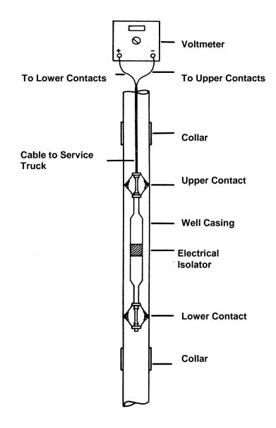
FIGURE A1—Casing Potential Profile Tool
