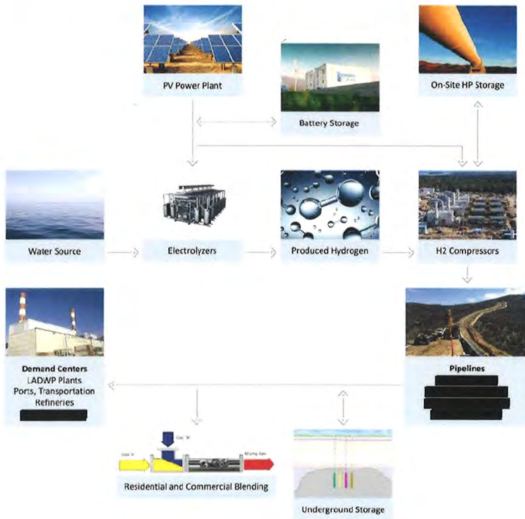
FIGURE 2A, SYSTEM 2: MOJAVE LOW DEMAND SCENARIO OVERALL FLOW DIAGRAM
