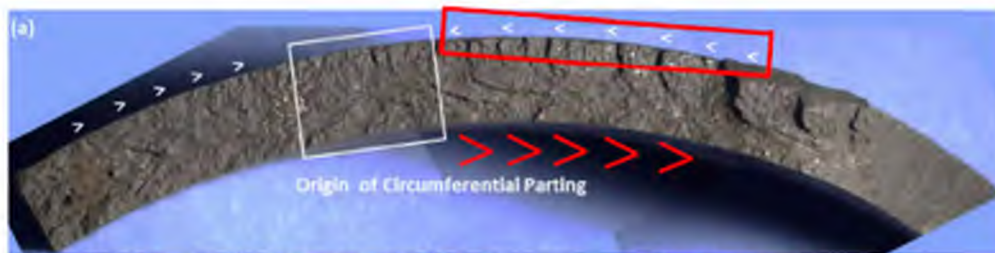
Figure 15. Figure 68 from page 72 of Blade main report. Red rectangle encloses backward chevron marks drawn by Blade. Red chevron marks inserted above are consistent with chevron marks present on the fracture surface. Blade misidentifies the chevron marks as flowing towards the origin. Based on both my physical inspection on February 27-28, 2020, and my analysis of this image, the chevron marks travel to the right, as indicated by the red arrows at the bottom of the figure.
