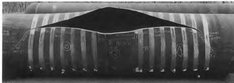
Fig. 1 Ductile fracture of a full section X60 grade line pipe tested at 56 °F (13 °C), which is 8 °F above its 50% shear-area DWT
