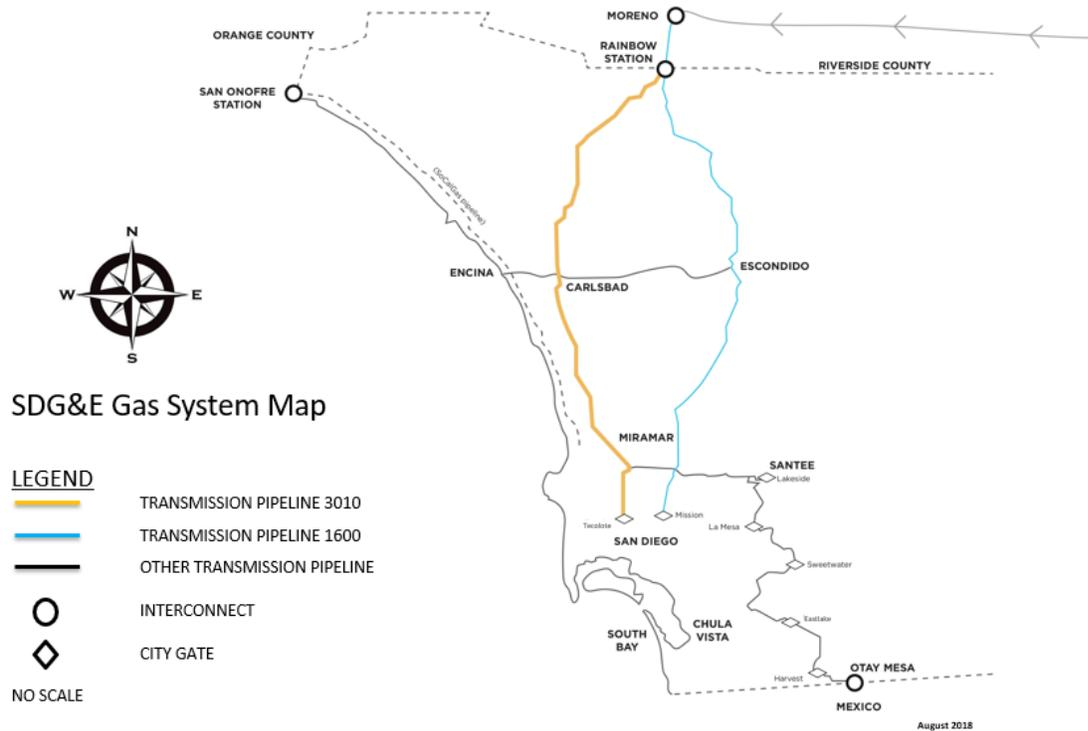
The SDG&E gas transmission system is designed to flow gas supplies from north to south, starting at the Riverside County line, and south to north, starting at the Mexican border, to meet consumer demand for heating homes on peak winter days, providing gas service to commercial and industrial operations, and to generate electricity to meet cooling demands on the hottest
